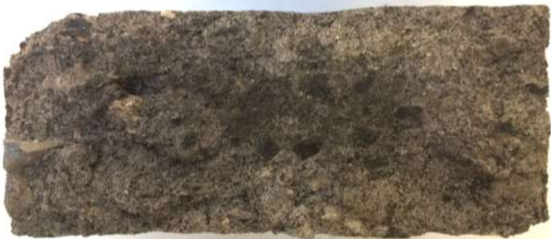
Figure 12. Cracked surface after ITS test on specimen obtained from L386
