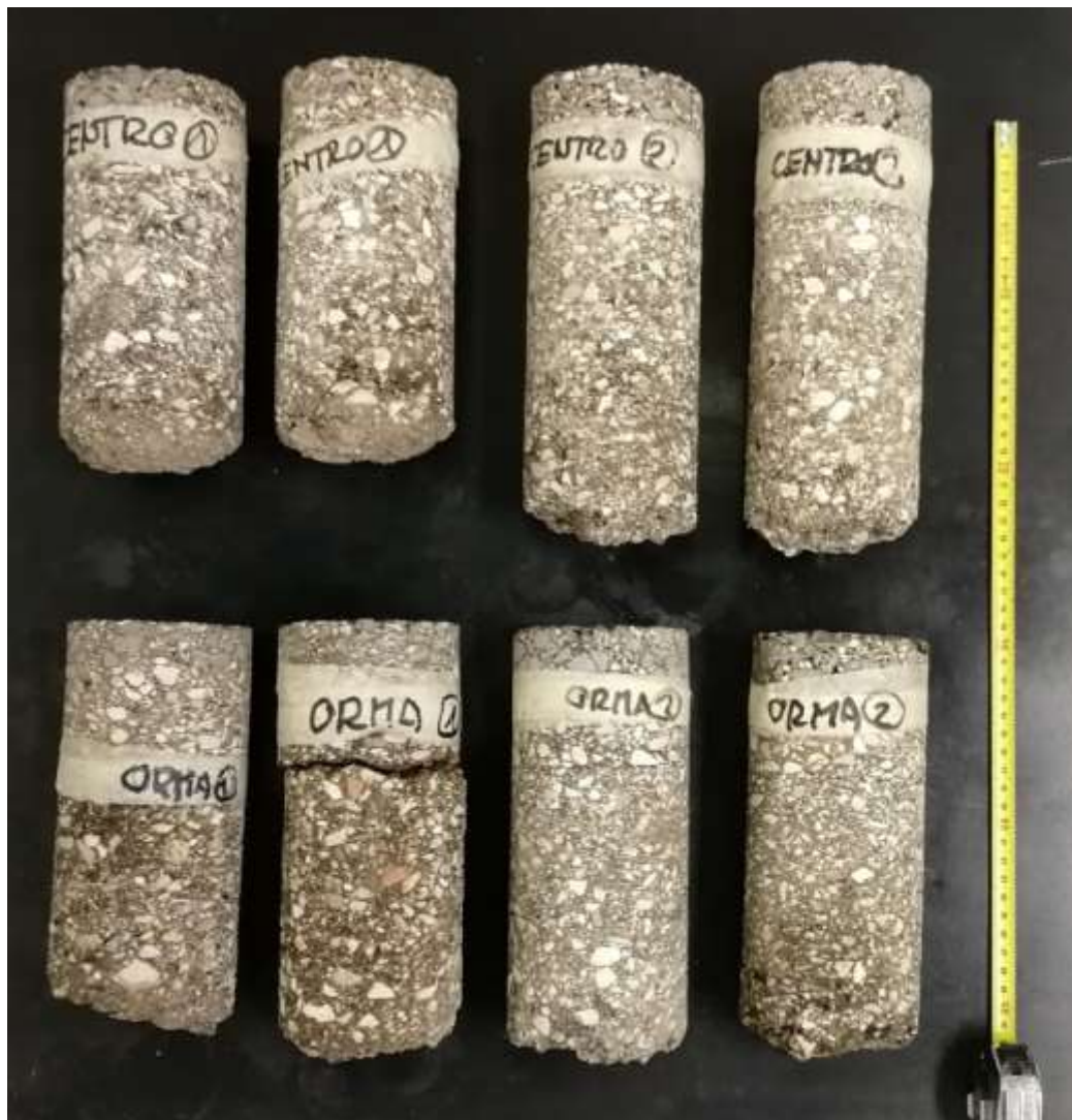
Figure 40: SP18 cores taken in October 2019. From the top-left, first row: C1.1, C1.2, C2.1, C2.2; second row: W1.1, W1.2, W2.1, W2.2
