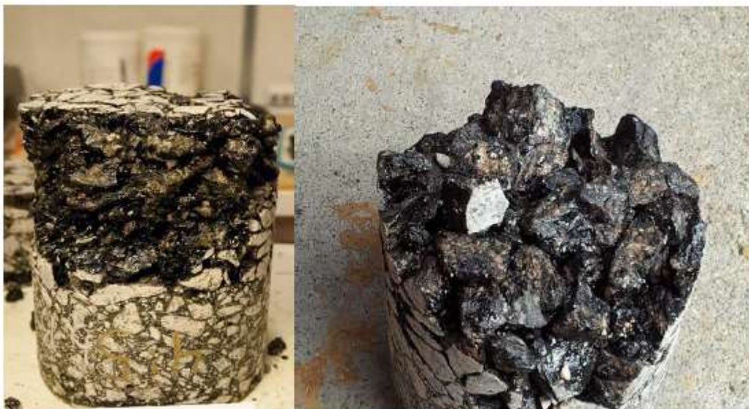
Core samples from the base layer with poor bitumen coverage.
