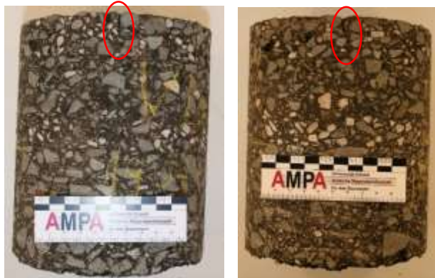
Figure 9. L386 cores extracted from cracked zones.
