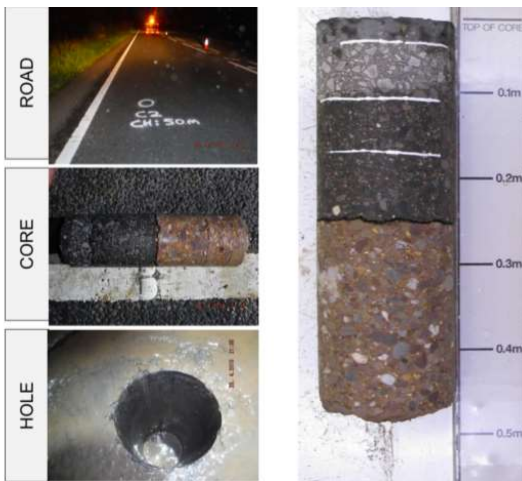
Figure 1 Coring procedures performed by AECOM UK
